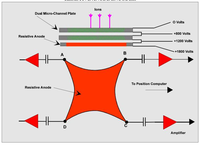
The pulses are amplified and passed to the position computer where the X and Y position is calculated by the equations:
