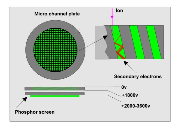
As with the discrete dynode electron multipliers, these micro-channel plates do discriminate according to the ion species, and over a period of time, the secondary electron gain is reduced. Under ideal operating conditions, a count rate of ~5000 c/s should be visible on the phosphor screen.
