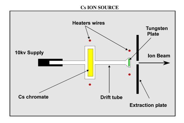
In the Cameca ims-series, Cs ion beams are generated by a surface ionisation process. Cs vapour is produced by the heating of a solid Cs compound (Cs-chromate or Cs-carbonate). The Cs vapour travels along the drift tube and strikes a tungsten plate where it is thermally ionised. Any atom or molecule coming from the reservoir is forced to bounce between the tungsten plate and the ioniser tip. This results in most atoms being ionised and escaping through the small hole in the cap.
