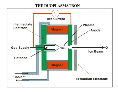
Many ion species are generated within the duoplasmatron and it is left to the primary beam mass filter to select the desired ion beam (Section 3).
