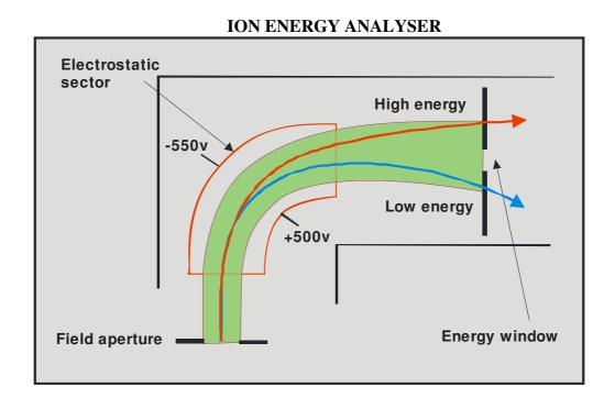
The inner and outer spherical electrode surfaces of the energy analyser have voltages of opposite polarity; which is positive and which negative depends on the polarity of the secondary ion beam.
