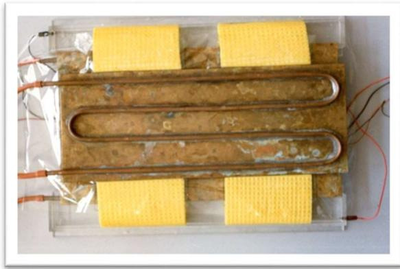
I then used sponge cloths to connect the buffer in the tanks to the surface of the gel. After covering the gel with clingfilm a second brass cooling plate was placed on top of the gel. The electrodes were connected to a power supply with the negative (cathode) terminal at the sample end of the gel and the positive (anode) terminal at the other end.
